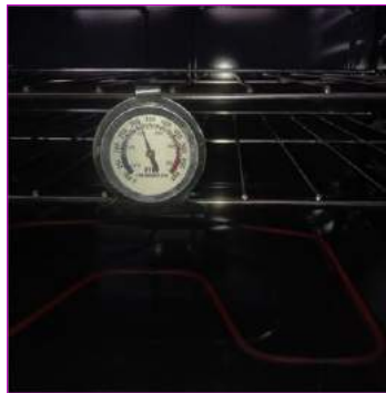
Oven temperature test 325° F
